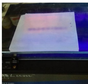
Figure 1: nitrocellulose membrane placed on UV to cross link the DNA.
