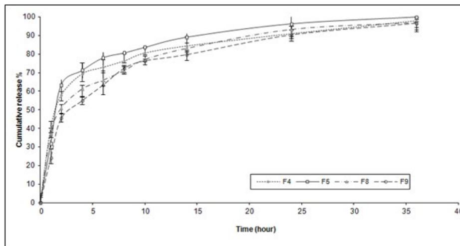
**Figure 3:** The in-vitro release profile of unPEGylated liposome (F4, F9) and PEGylated liposomes (F5, F9) in PBS medium at 37°C.
