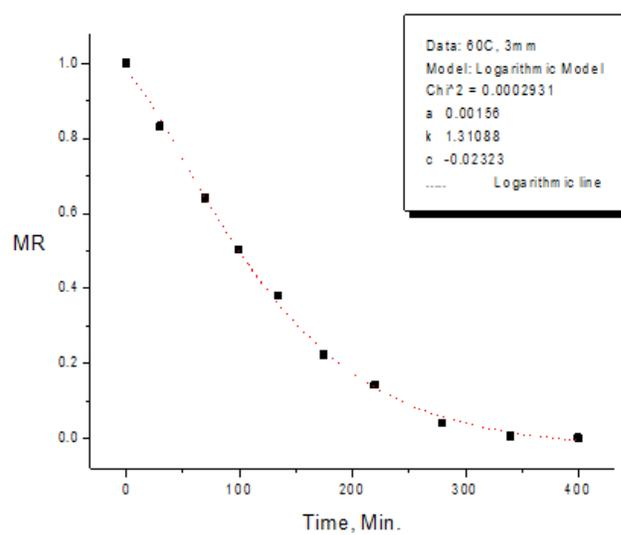
**Figure 8:** Variation in Moisture Ratio with drying time (60 °C, 3 mm thickness).
