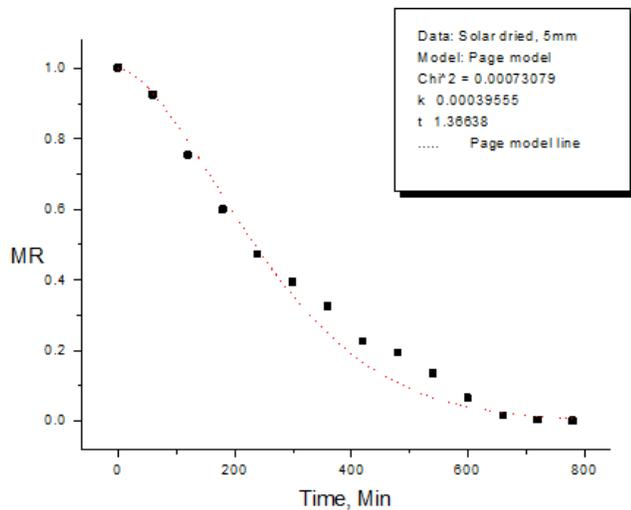
**Figure 15:** Variation in Moisture Ratio with time (Solar dried, 5mm thickness).
