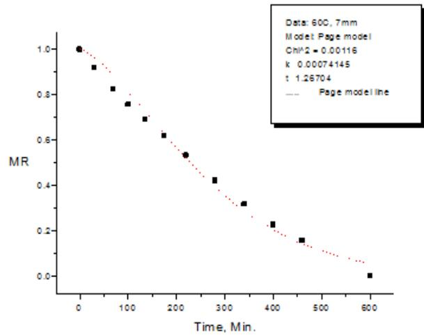
Figure 10: Variation in Moisture Ratio with drying time (60 °C, 7 mm thickness).
