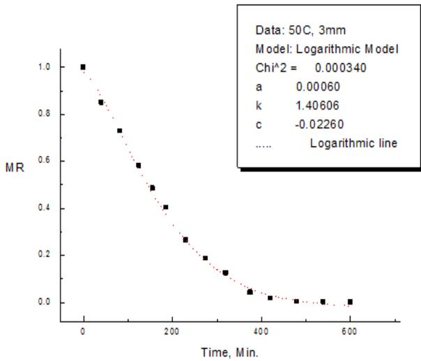
**Figure 5:** Variation in Moisture Ratio with drying time (50 °C, 3 mm thickness).
