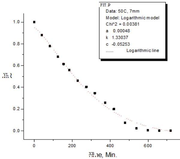
**Figure 7:** Variation in Moisture Ratio with drying time (50 °C, 7 mm thickness).
