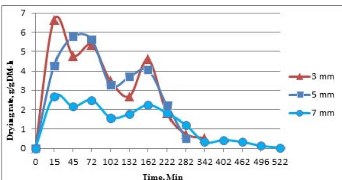
**Figure 3:** Variation in drying rate with time (70 °C Air temperature).
