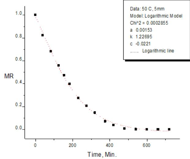
**Figure 6:** Variation in Moisture Ratio with drying time (50 °C, 5 mm thickness).
