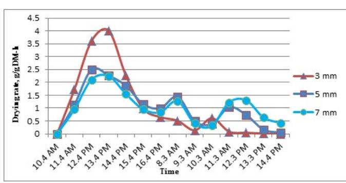
**Figure 4:** Variation in drying rate with time (Solar dried).
