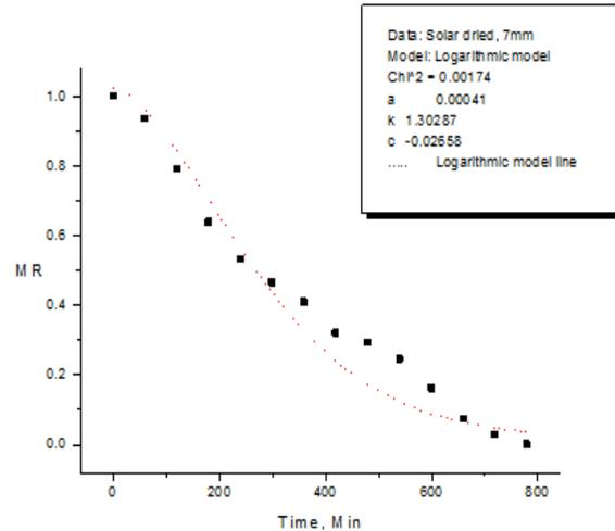
**Figure 16:** Variation in Moisture Ratio with time (Solar dried, 7mm thickness).
