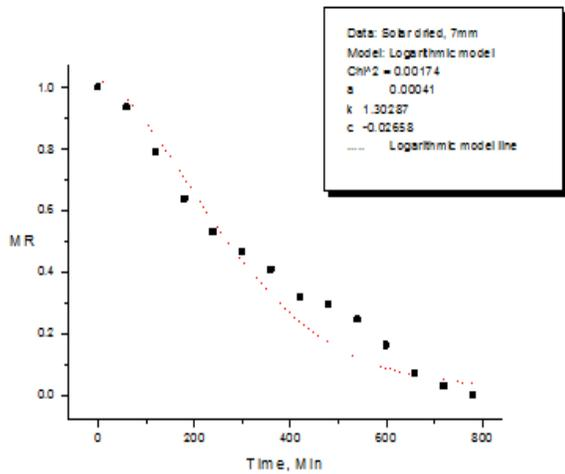
Figure 11: Variation in Moisture Ratio with time (Solar dried, 7mm thickness).
