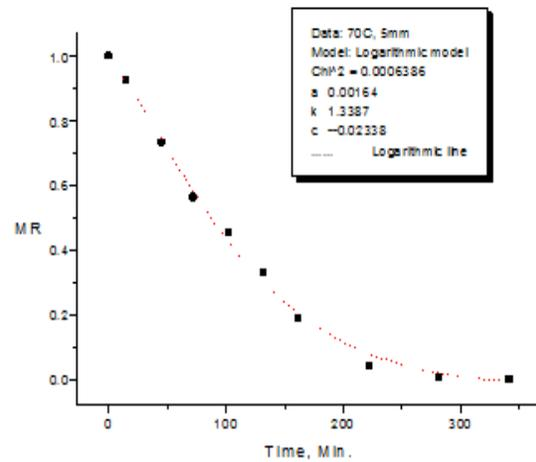
Figure 12: Variation in Moisture Ratio with drying time (70 °C, 5 mm thickness).
