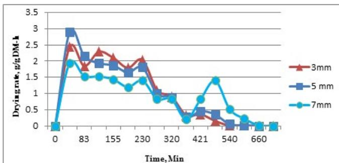
**Figure 1:** Variation in drying rate with time (50 °C Air temperature).
