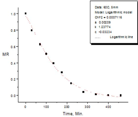
Figure 9: Variation in Moisture Ratio with drying time (60 °C, 5 mm thickness).
