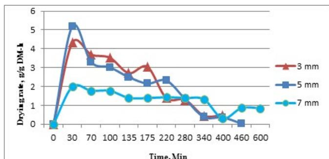
**Figure 2:** Variation in drying rate with time (60 °C Air temperature).
