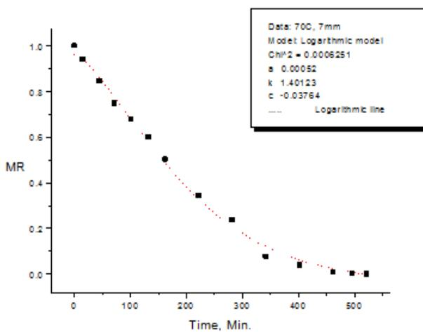
Figure 13: Variation in Moisture Ratio with drying time (70 °C, 7 mm thickness).
